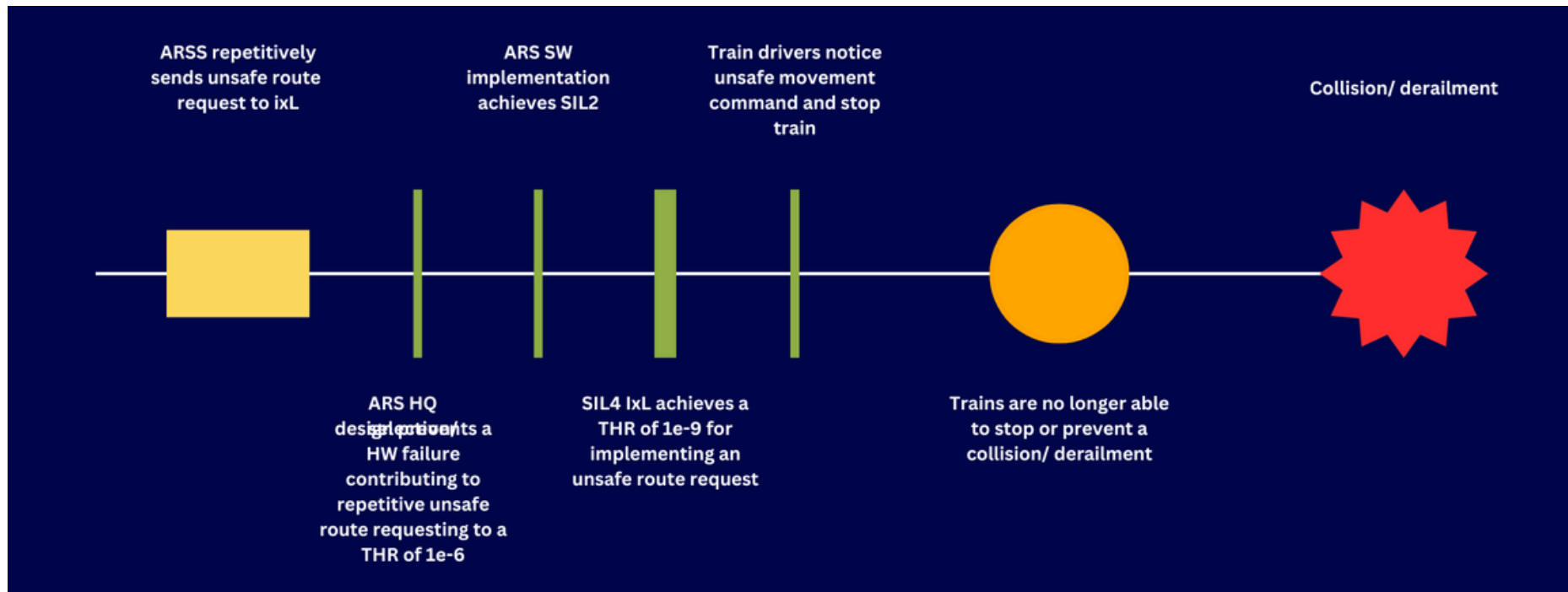
Fig. 5: Simplified ARS Threat Barrier Diagram
